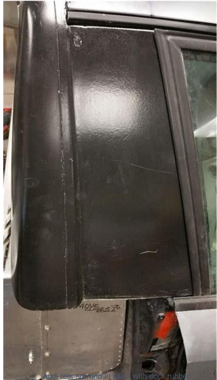
Audi rear surround in place with door rubber
