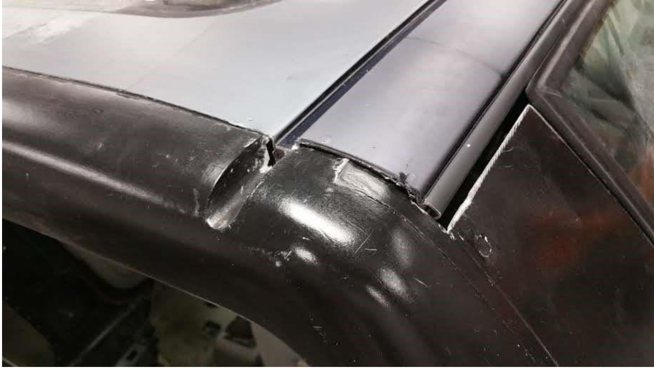
Audi top of rear surround in place
