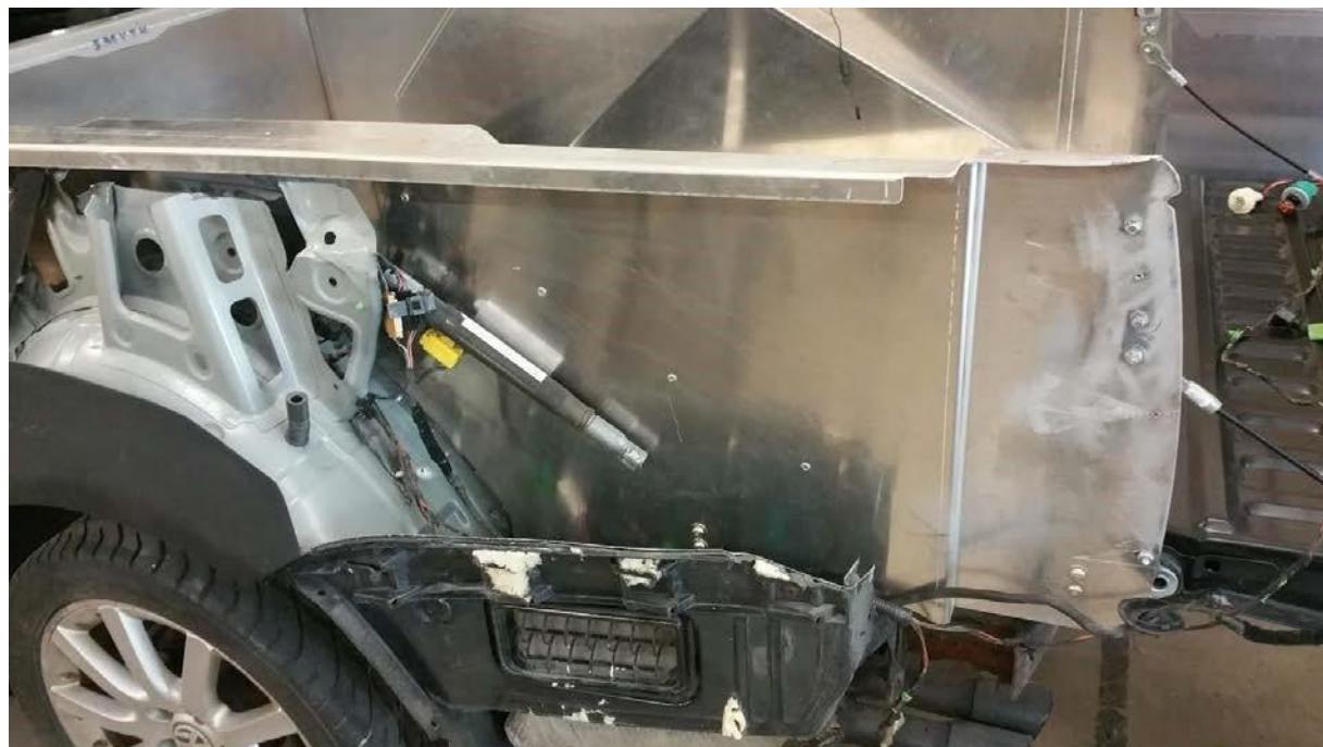
In this view above of the mk5 you can see that we mounted the airbag cylinder in the rear and left it wired...no rear passengers so the cylinder vents to the outside and no error lights on the dash.
