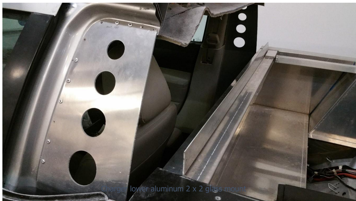
Charger rear surround is different as it assembles in 3 pieces, two sides and a top(see video)
