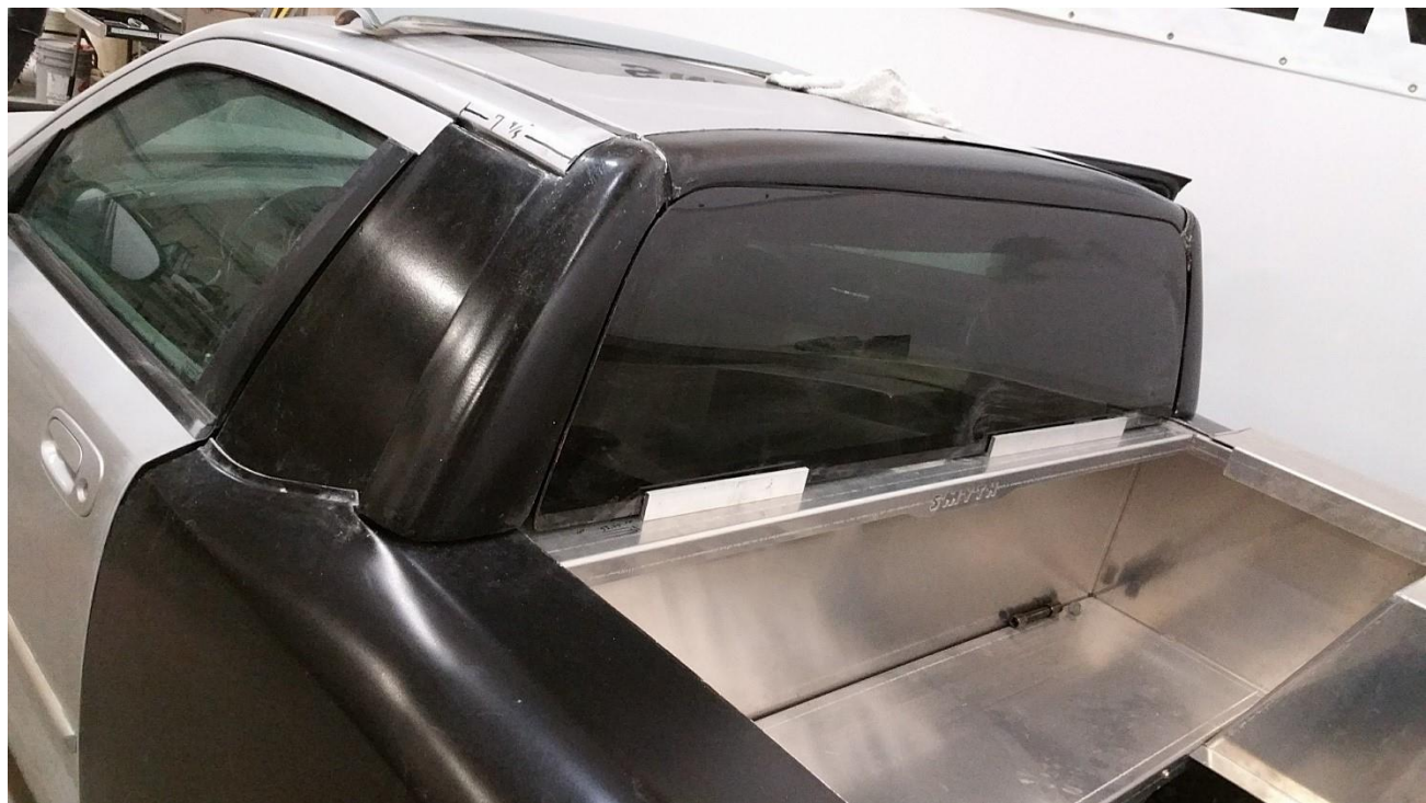
Charger rear surround is different as it assembles in 3 pieces, two sides and a top(see video)
